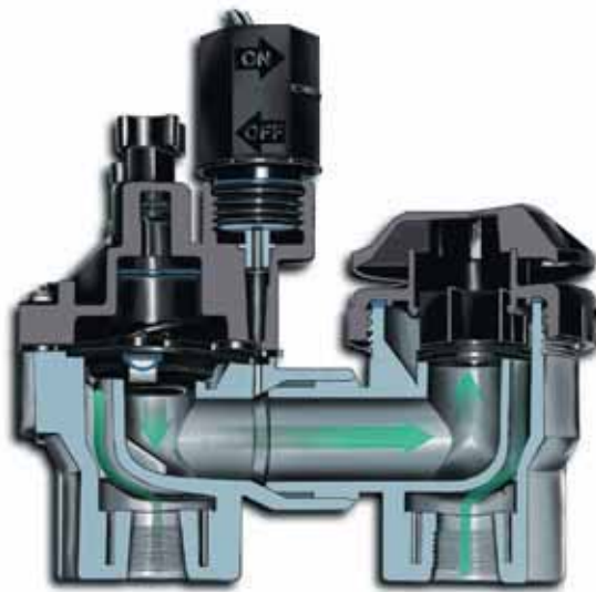
ASVF Cutaway
